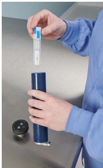
Figure 2: Specialized test pack designed for 10-minute prevac cycles operating at 270°F.
