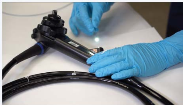
Figure 1: Borescope insertion for visualization of residual moisture within an endoscope channel
