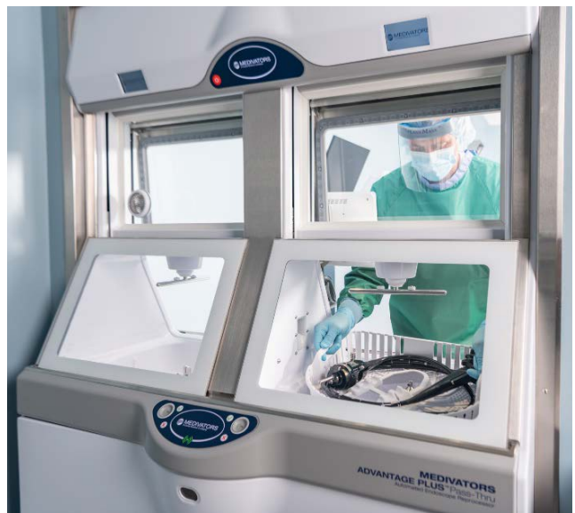
Figure 1 Pass thru automated systems give separation between loading of the cleaned endoscopes in decontamination and unloading of processed endoscopes on the clean side of the wall.
