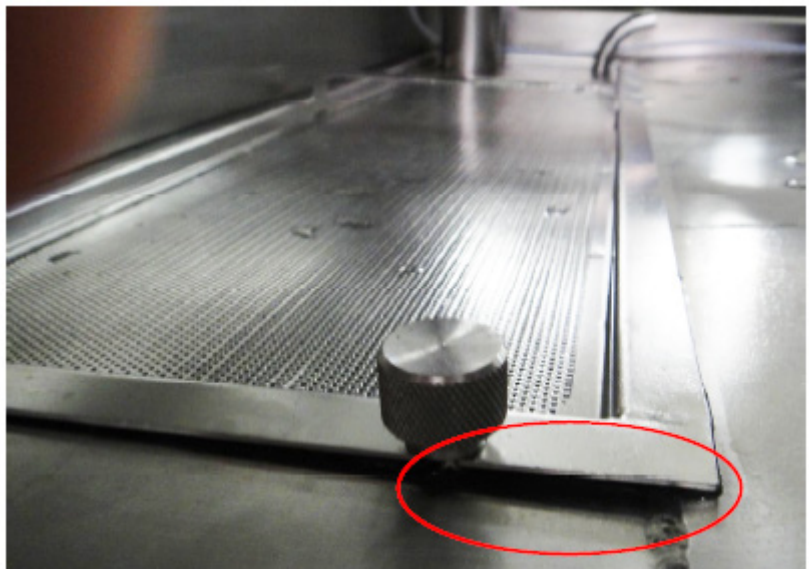
Figure 4: Washer debris screen installed incorrectly.
