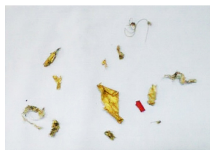
Figure 3: Example of debris found inside washer's rotatory arm. Tape, plastic markers, human hair, and other.
