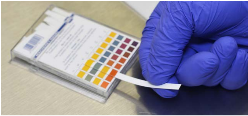
Figure 1: Test strips are available for routine monitoring of pH, water hardness, and some chemical impurities found in water.
