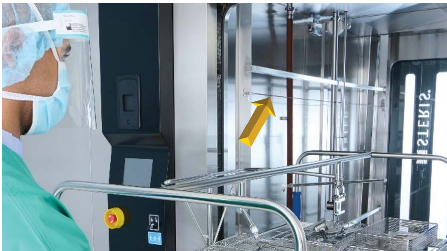
Figure 2: Arrow showing location of kill cord in cart washer.
